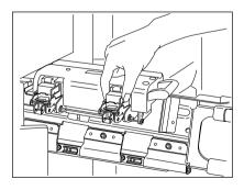
While pushing down on level ①, pull up knob ②.
